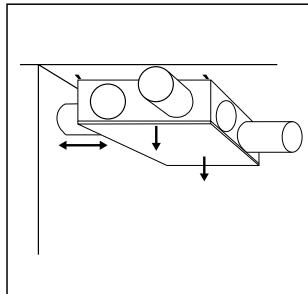
Make sure that the wall or the ceiling to which the fan will be fixed, is strong enough to support the weight of the fan. (18 kg i.e. more than 4.5 kg at each fixing).
