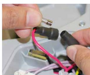
5. Unscrew the fuse holder and replace with a new **fuse 5x20mm, delayed: class T, 200mA, 250V**.
