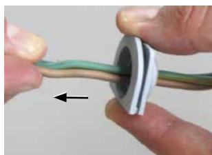
8. Thread the cable-shifter on the feeder (feeder not provided).
