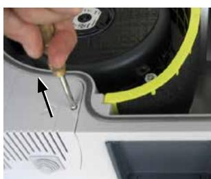
3. Unscrew (1 screw) and withdraw the trap door of the electrical case.
