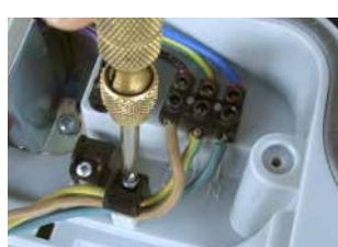
10. Block the cable in the cleat and thread the cable-shifter in the lid of the case.
