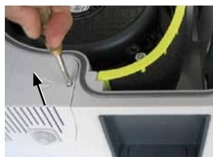
7. Unscrew the lid of the electrical case by using a PH1 screwdriver.
